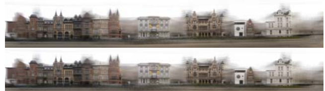
Figure 7 First row: the average image of all the projected sources for the scene shown in Figure 1. Notice that the street curves up towards the right. Second row: the average image after unwarping to straighten the ground plane and cropping.
