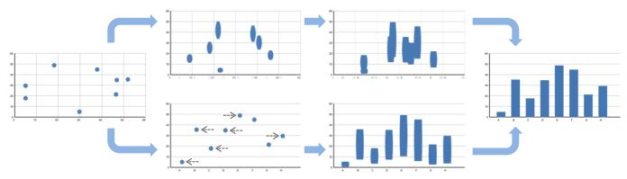
**Figure 1. Animating from a scatter plot to a bar chart.** The top path directly interpolates between the starting and ending states. The bottom path is staged: the first stage moves points to their x-coordinates and updates the x-axis, the second stage morphs the points into bars.
