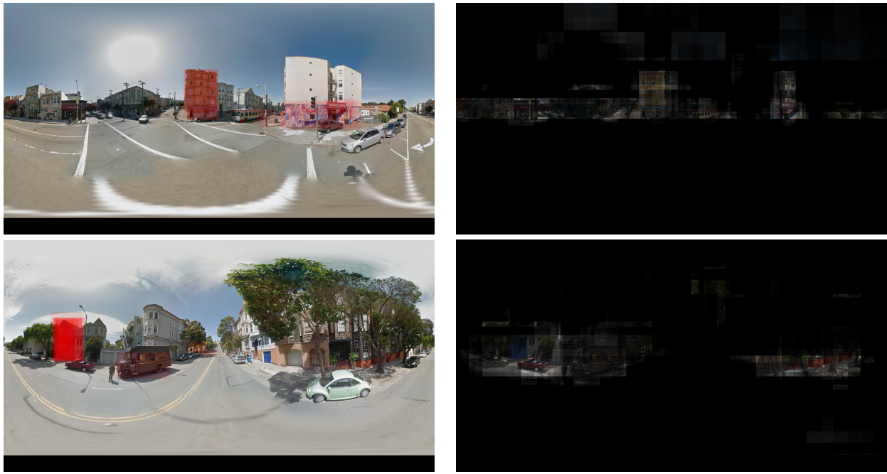
Figure 7: A comparison of a success case (top) and a failure case (bottom). Notice that the model is capable of picking out buildings that colored significantly different, except in the presence of distracting objects (cars, people, etc). We hope to remedy these shortcomings by eliminating these superfluous elements as a pre-process.
