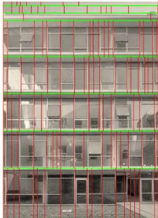
Figure 14: The tile segmentation is poor because of the small margin between windows and the glare created
