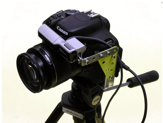
Figure 5. DSLR with attached webcam.
