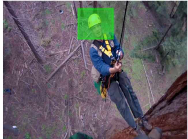
Figure 10. Selecting a rectangular region in the image can unintentionally force input frames to match the background included in the marquee region, even if only the helmet in the foreground was intended.
