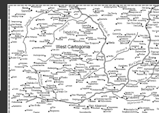
Cartographer Eduard Imhof's labeling heuristics transformed into penalty functions for an optimization based point labeling system [Edmondson 97]
