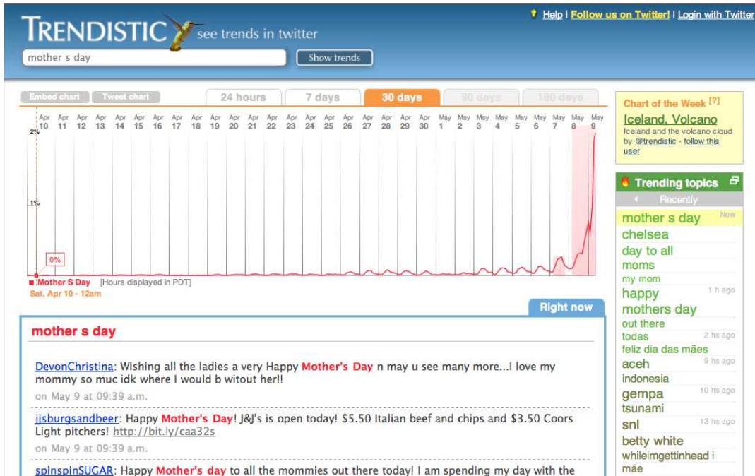
Fig. 3. Trendistic - A current implementation of twitter trend statistics. This system focuses on a single trend and plotting its pertinent tweets and statistics. It does not update automatically (requires refresh). It lists other popular trends in a box on the right side of the screen.
